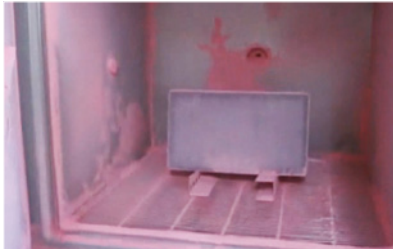
Test for protection against dust
