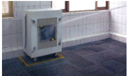
IEI's LCD products are front sealed and tested in the certified house chamber under UL's Witnessed Test Data Program (WTDP).
